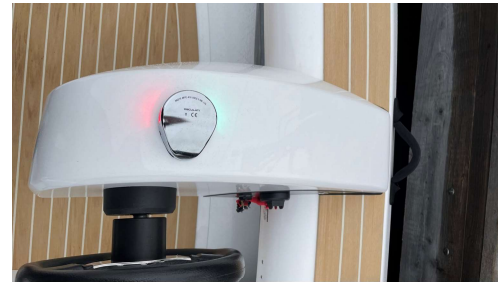
Installed nav lights
